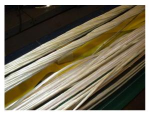
Figure 2- Rifled Core Yarns vs Parallel
