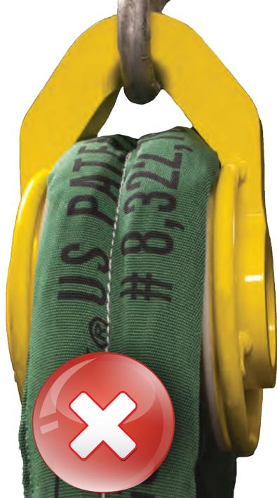
Do not use a Twin-Path® Sling that is wider than the footprint of the Synthetic Equalizer Block sheave.
