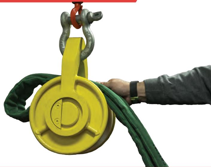
Flatten the body of the Twin-Path® Sling.
