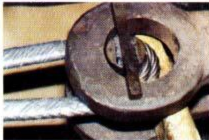
Photo #10 Positioning of dual loops of wire rope for pin test
