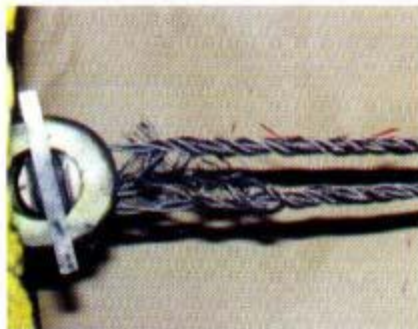
Photo #6 Wire rope rupture in pin test - 4/ D/d ratio
