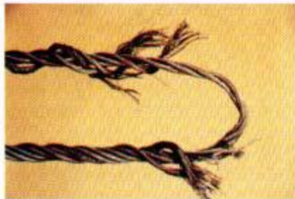
Photo #7 Failure location of wire rope in pin test at pin contact
