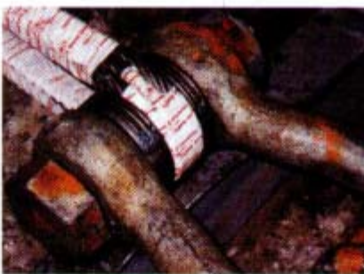
Photo #4 Ultimate tensile testing of Gator-Max® sling - 1/1 D/d ratio)
