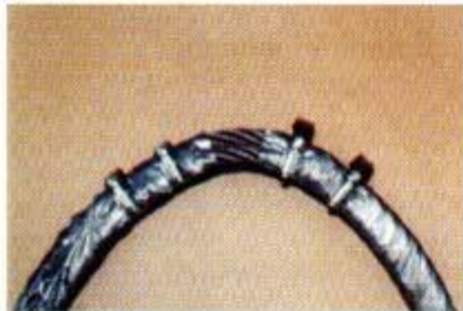
Photo #9 Dual loops with tape & u-bolts for pin testing
