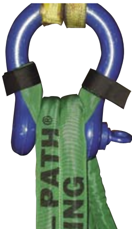
Sling protection at the pin connection point helps prevent slings from becoming cut.
