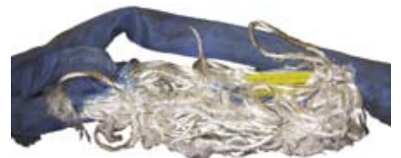
This shows a sling failure due to stitching that punctured core yarns.
