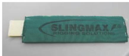
Pictured above is yellow 9800GN nylon web sling material protected by Slingmax® Covermax® roundsling tubing. The exposed webbing faded to white after 334 hours of UV exposure. When the nylon web was pulled out of the protective Slingmax® cover, you can see the original yellow color remains. It shows no UV degradation to the protected webbing.
