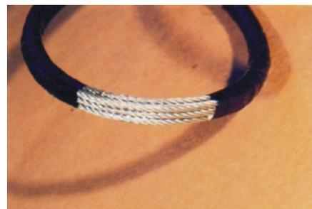
12-part "parallel laid" eye on a Gator-Max sling.
