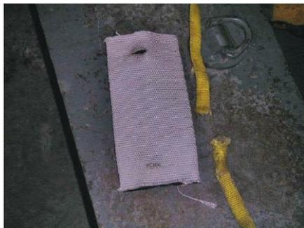
**Pads used for abrasion protection were long thought to also provide cut protection. Recent testing has proven this theory wrong, and dangerous.**
