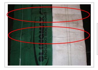
No damage was found on the Cornermax<sup>®</sup>/Dyneema<sup>®</sup> Sleeve after this test.
