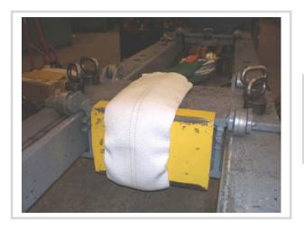
The 10" Cornermax®/Dyneema® Sleeve was placed over a TPXC 15,000 and pulled over the 90° edges of a sharpened steel plate.
