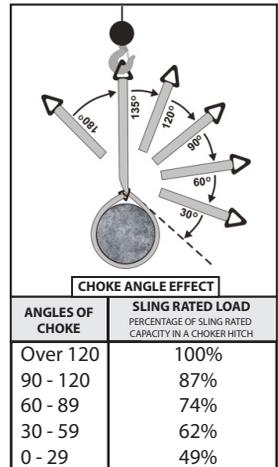
⚠ Use caution with lifts at angles less than 45° and do not make lifts with slings at less than 30°. When possible, use longer slings to minimize angular tension by increasing the angle. Severe angles can greatly reduce sling strength.
