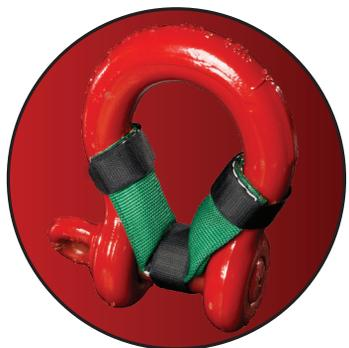
**Synthetic Armor** Pads protect slings from abrasion damage that can be caused by contact with rough surfaces such as concrete beams and structures. They are also used to protect finished or painted loads from marring. Synthetic Armor can be made to fit any length or width sling.
