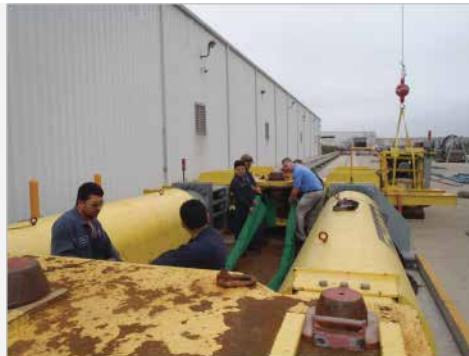
3,000,000 lbs. Twin-Path® sling test
