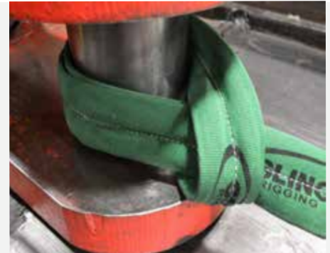
Check-Fast® System functionality in different hitch configurations
