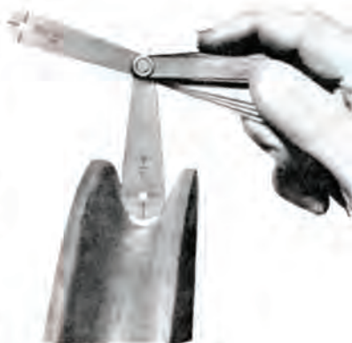
Photo shows new gauge and worn sheave. This new gauge is designed with one-half the allowable oversize (see table). Using the new gauge, when you do not see light, the sheave is OK. When you do see light under the new gauge, the sheave should be replaced.
