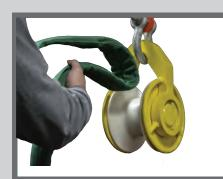
The Equalizer Block is used to maintain tension on all legs of the sling during a lift. Rather than adjusting slings and hooks prior to completing a lift, the Equalizer Block will automatically adjust itself when load is put on the device from the sling.
