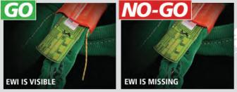
All Twin-Path<sup>®</sup> slings are equipped with the Check-Fast<sup>®</sup> Inspection System to assist with the sling inspection process. The Check-Fast<sup>®</sup> External Warning Indicator (EWI) provides a criteria for a pass/fail inspection and can detect severe overload, UV light degradation, fiber on fiber abrasion and overall sling fatigue.
