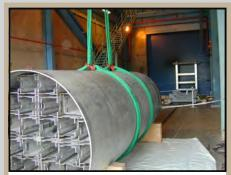
Reliability in the manufacturing process. Twin-Path<sup>®</sup> slings have been cycle tested to over 50,000 cycles. Rifled Cover Technology<sup>®</sup> ensures that the sling fibers are seeing equal load, and the redundant Twin-Path<sup>®</sup> design provides an extra level of safety.
