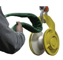
Flatten the body of the **Twin-Path Sling**
