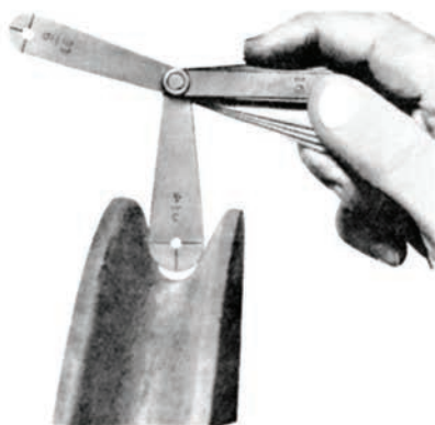
Photo shows new gauge and worn sheave. This new gauge is designed with one-half the allowable oversize (see table). Using the new gauge, when you do not see light, the sheave is OK. When you do see light under the new gauge, the sheave should be replaced.
