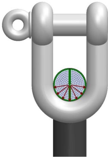
TAPERED SLING IN HARDWARE THAT SUPPORTS THE TAPERED DIAMETER
