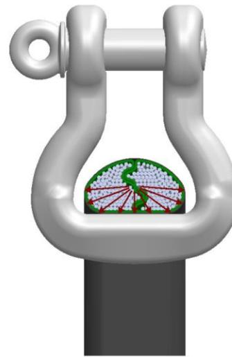
TAPERED SLING IN HARDWARE THAT DOES NOT SUPPORT THE TAPERED DIAMETER
