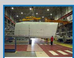
Reliability in the manufacturing process. Twin-Path® slings have been cycle tested to over 50,000 cycles. Rifled Cover Technology® ensures that the sling fibers are seeing equal load, and the redundant Twin-Path® design provides an extra level of safety.
