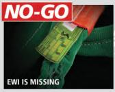
All Twin-Path® slings are equipped with the Check-Fast® Inspection System to assist with the sling inspection process. The Check-Fast® External Warning Indicator (EWI) provides a criteria for a pass/fail inspection and can detect severe overload, UV light degradation, fiber on fiber abrasion and overall sling fatigue.
