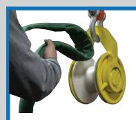
The Equalizer Block is used to maintain tension on all legs of the sling during a lift. Rather than adjusting slings and hooks prior to completing a lift, the Equalizer Block will automatically adjust itself when load is put on the device from the sling.
