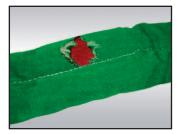
The separate inner cover shows red for warning that the sling is damaged and should be taken out of service.
