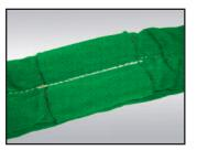
Twin-Path® slings are repaired with patches like this. Each sling is proof tested after a repair.
